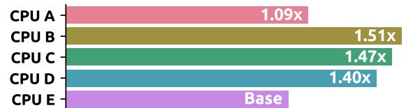
Fig. 9. Relative SDC rate of the five microarchitectures. The same DPPM is used across CPUs to only highlight intrinsic differences.
