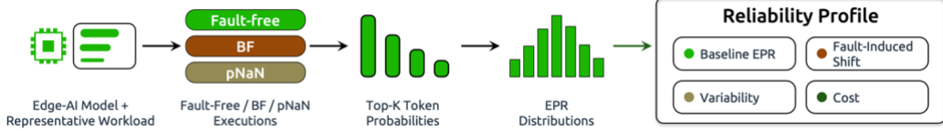
Figure 1: Edge-AI reliability-profiling workflow. Fault-free and corrupted executions produce token-probability traces from which EPR distributions are obtained to characterize baseline behavior, corruption-induced displacement, variability, and measurement cost for each model-workload pair.
